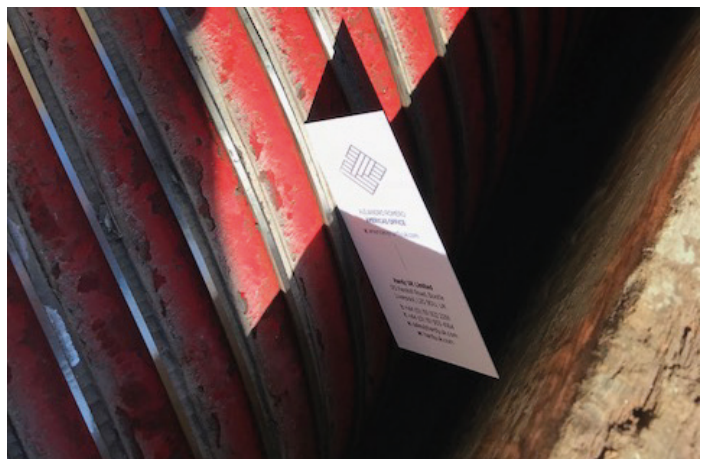
Business Card Used to Highlight Space Between Caulking and Blade
