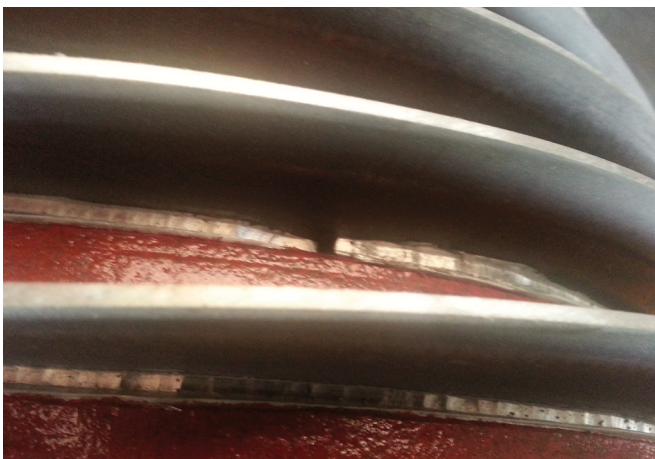
Cracked Aluminium Caulking
